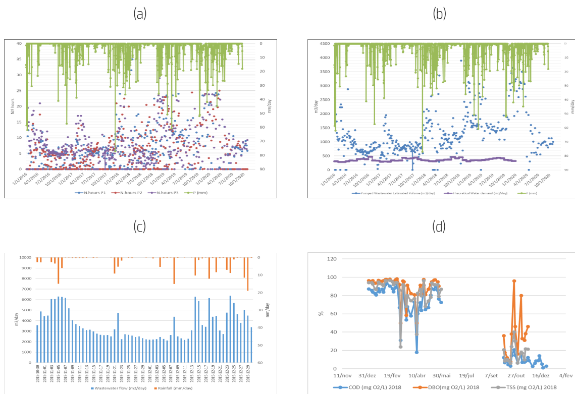
Figure 1: (a) Pump station hour analysis vs rainfall; (b) Estimated pump flow vs rainfall; (c) WW Event infiltration decay analysis (30/10/2015 - 30/12/2015); (d) WW WRRF treatment minimum efficiency
