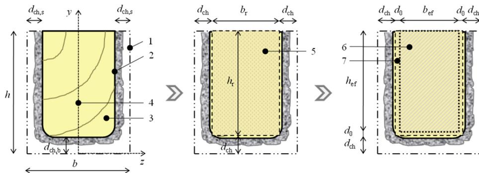
Figure 1: Schematic of the reduced cross-section method. 1 Initial cross-section; 2 Charring line; 3 Residual cross-section with rounding; 4 Coordinate system; 5 Rectangular residual cross-section; 6 Effective cross-section; 7 ZSL [8].
