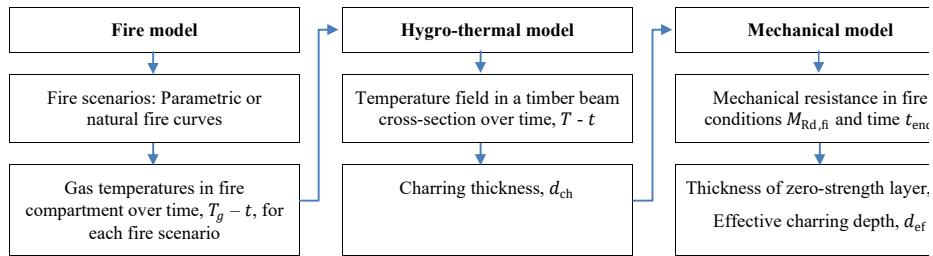
Figure 3: Schematic of sequentially performed analyses by means of the fire, the hygro-thermal, and the mechanical models and the outcomes used in [7, 8, 9].
