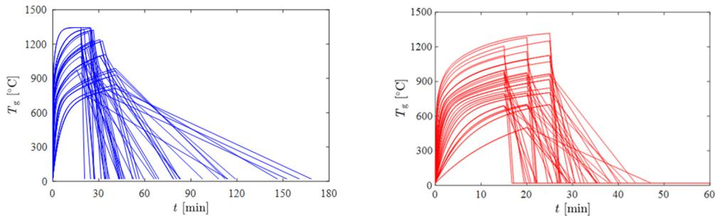
Figure 4: On the left different ventilation controlled parametric fire curves in considered [7] and on the right fuel controlled parametric fire curves [8].
