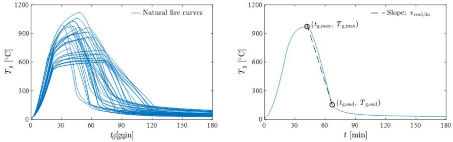
Figure 7: Modelled 44 fire scenarios, i.e., natural fire curves (left) and symbols of a natural fire curve for specific fire scenario (right) [9].
