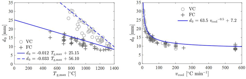
Figure 6: Expressions for the ZSL thickness  $d_0$  depending on parameters  $T_{g,max}$  (left) and  $v_{cool}$  (right) [8].
