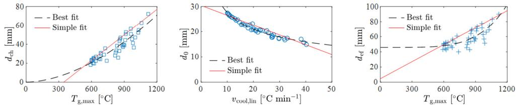
Figure 8: The charring thickness  $d_{ch}$ , the zero-strength layer thickness  $d_0$  and the effective thickness  $d_{eff}$  at the time  $t_{end}$  in relation to  $T_{g,max}$  (left),  $v_{cool}$  (middle) and  $T_{g,max}$  (left), [9].
