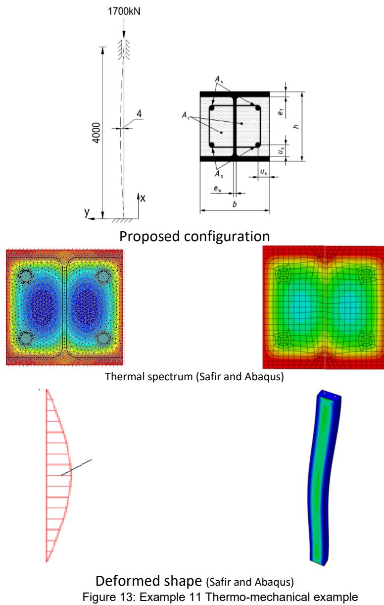
Figure 13: Example 11 Thermo-mechanical example
