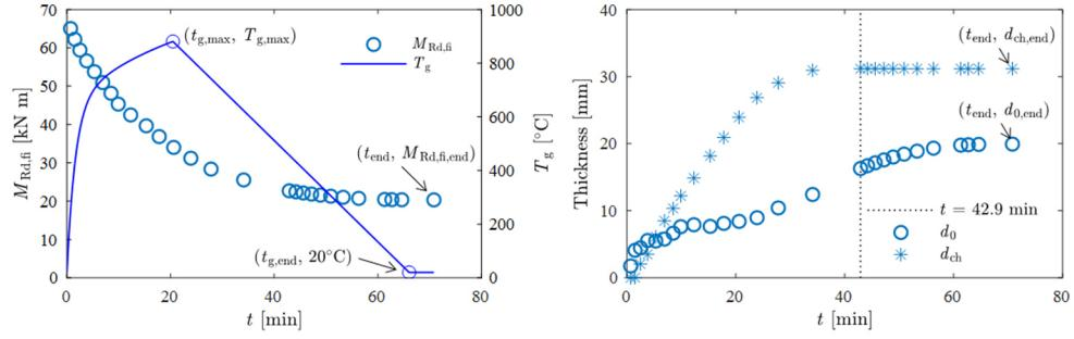
Figure 5: The development of  $M_{Rd,fi}$ , and  $T_g$ , over time (left) and developments  $d_{ch}$  and  $d_0$  over time (right) [7].
