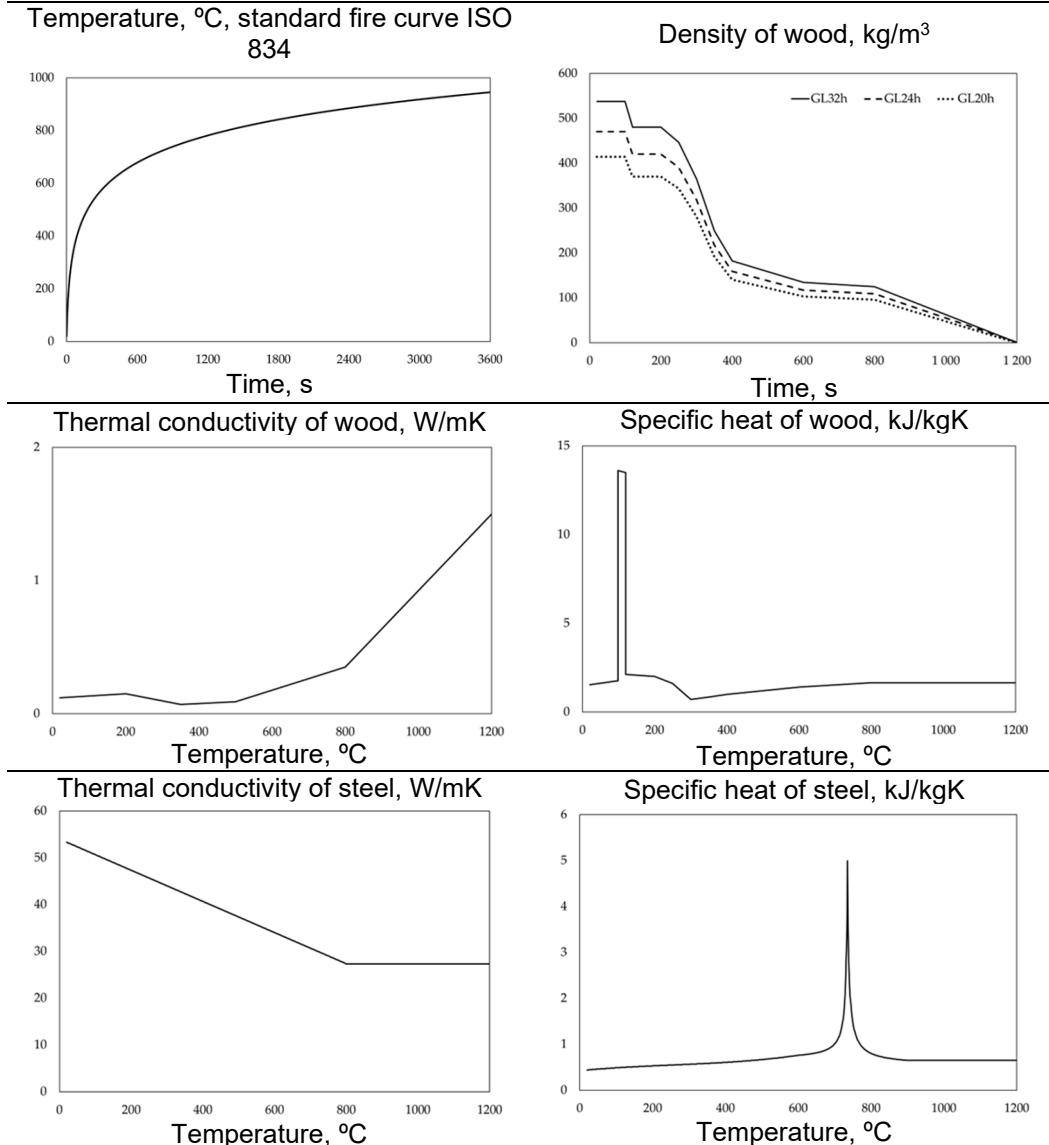
Figure 3: Time fire curve and thermal material properties of wood and steel.
