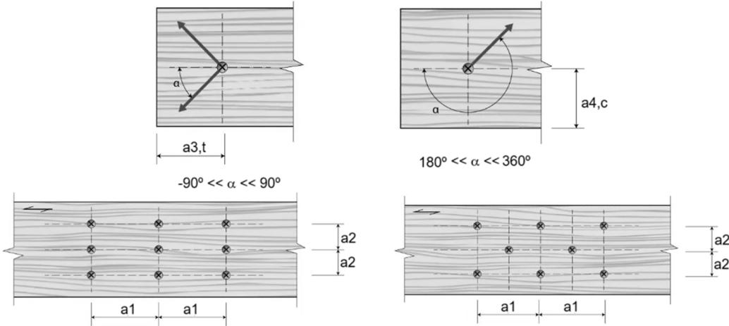
Figure 5: Spacing or edge/end distance between dowels in connections.
