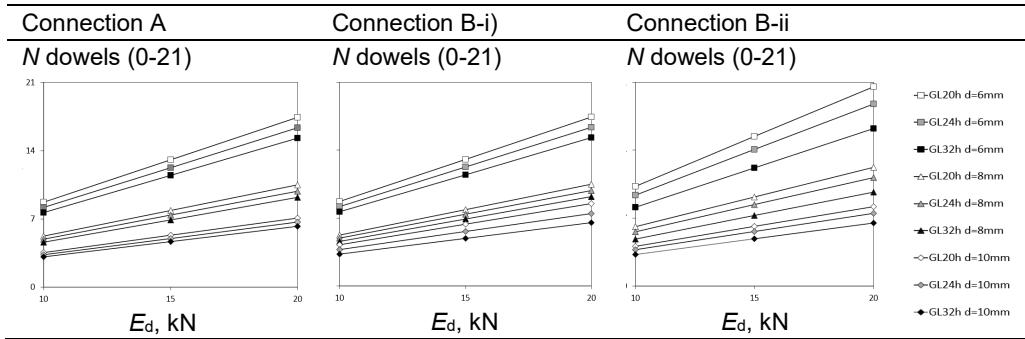
Figure 4: Number of dowels for fasteners in single shear.
