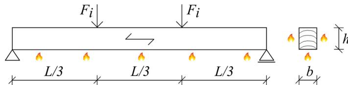
Figure 2: Schematic of the analysed simply supported timber beam in studies [7, 8, 9].
