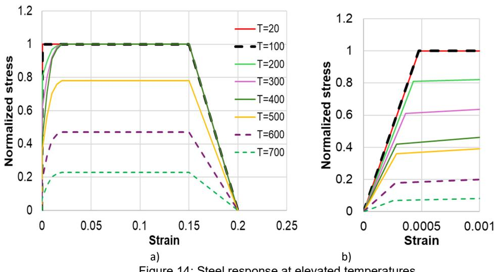
Figure 14: Steel response at elevated temperatures
